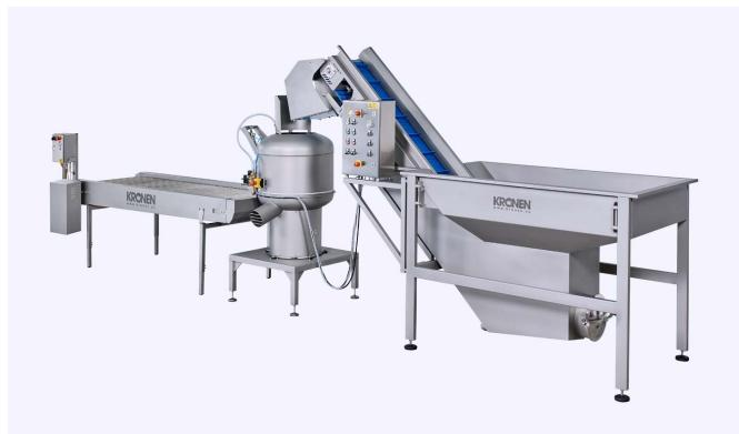
peeling machine can be transformed into a practical washing machine for tuber vegetables within three minutes.
