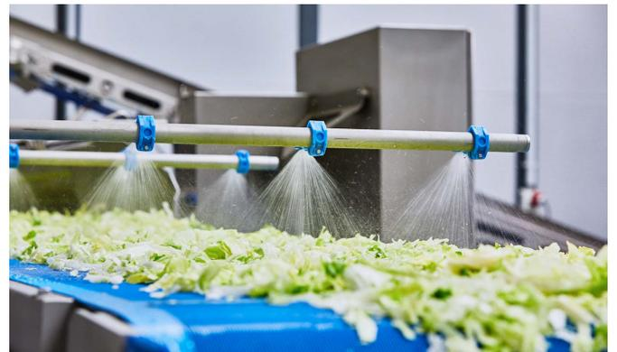
outfeed by means of an overflow and sprayed with a fresh water shower. The water flows through a strainer into the pump tank, from which it is pumped back into the wash tank and used again.
